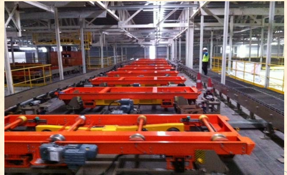
* Skillet conveyor installation with structure Fabrication Erection and Painting
